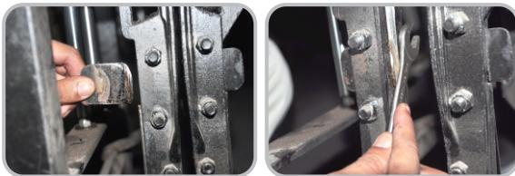
Checking Surface of cutter
